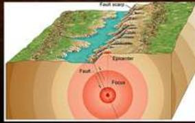
The diagram illustrates the mechanics of an earthquake. It shows a cross-section of the Earth's crust with a fault line. The point where the rupture begins is labeled 'Focus', and the point on the surface directly above it is labeled 'Epicenter'. The fault line is labeled 'Fault'.
